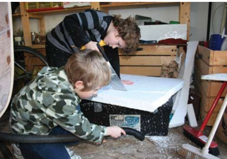
Above: Right way up at last, the Limpet awaits her rubbing strakes. Below left: Brendan cuts out the polystyrene pads which will add buoyancy to the undersides of the seat tops and Aidan cleans up after him. Below right: Brendan checks the shape of a quarter knee.
