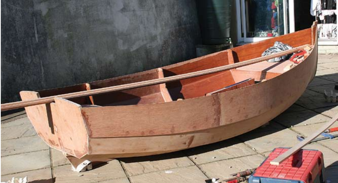
Above: Right way up at last, the Limpet awaits her rubbing strakes. Below left: Brendan cuts out the polystyrene pads which will add buoyancy to the undersides of the seat tops and Aidan cleans up after him. Below right: Brendan checks the shape of a quarter knee.
