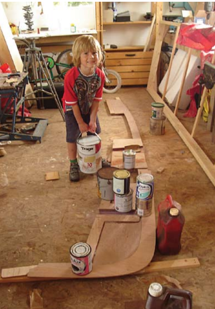
Left: The spine is strengthened by doublers epoxied in place. Right: Painting the daggerboard case and mast slot before assembly.
