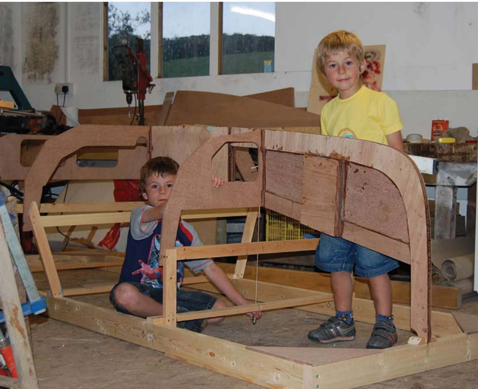
The packing case in which the Limpet kit arrives provides a good sturdy base for the building jig. Brendan checks the frames are vertical.
